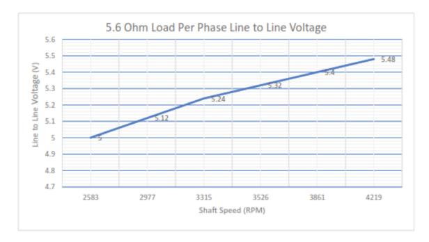
Figure 5: Terminal Voltage with 5.6 Ohm Star Connected Load
